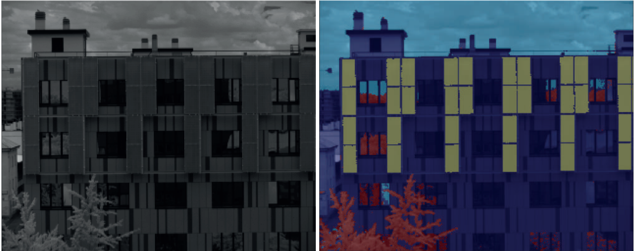
Example of Hyperspectral Imaging for remote sensing. The image on the right is the result of a classification algorithm, which distinguishes the sky (light blue), the buildings (purple), the tree (and their reflections in the windows of the building, in red) and the solar panels (in yellow).
